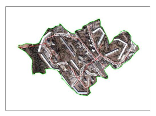
Figure 8. Medium-density catchment area (Pihlajamäki)\_in an urban/suburban area in the City of Helsinki. In this figure green line indicates the border of the catchment. Red lines illustrate the main stormwater pipeline system.
