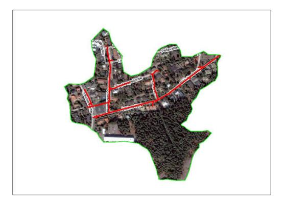
Figure 7. Low-density catchment area (Veräjämäki) in a suburban area in the City of Helsinki. The catchment border is illustrated by a green line. Red lines illustrate the main stormwater sewer pipeline system.
