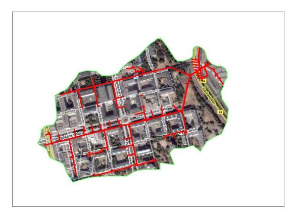
Figure 9. High-density catchment area (Itä-Pasila) in the core urban areas in the City of Helsinki. Green line indicates the border of the catchment. Red lines illustrate the main stormwater pipeline system.
